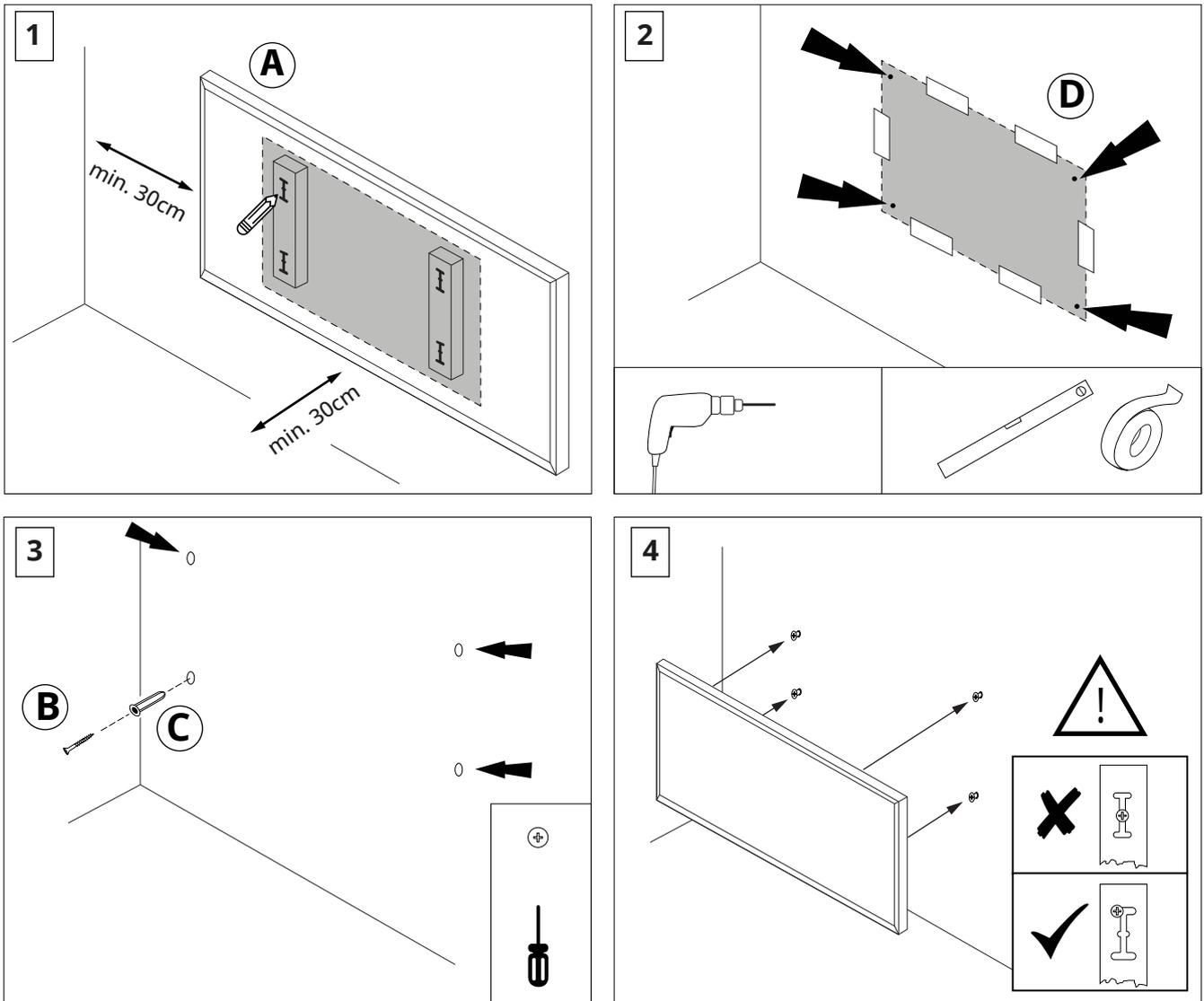
1. Use the supplied paper to cover the back of the panel, and use a pencil to mark the locations of the holes.
